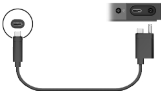
Figure 6. HP Elite Dock with Thunderbolt 3 cable
